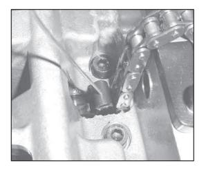
7. Allow three to four chain links to fall past the cylinder head parting line.
