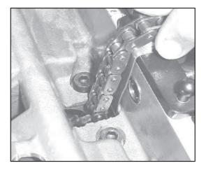
6. Insert the stuffer end of the Timing Chain Hook / Stuffer, PN-PW-47108, tool into the chain gallery.
