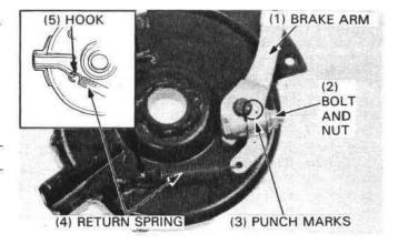
Install the brake panel on the knuckle.
