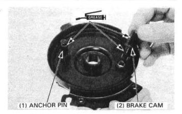
Soak the felt seal in clean engine oil and install the seal on the brake cam.
