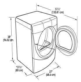
\*Most installations require a minimum 5" (12.7 cm) clearance behind the dryer for the exhaust vent with elbow. See Venting Requirements.
