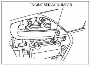
The engine serial number is stamped on the left side of the rear crankcase.
