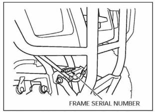
The frame serial number is stamped on the front side of the frame.
