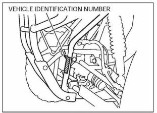
The Vehicle Identification Number (VIN) is located on the left side frame down tube.
