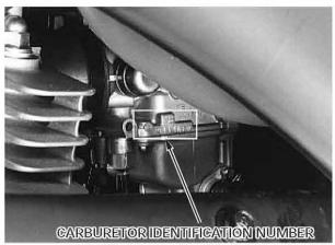
The carburetor identification number is stamped on the left side of the carburetor body.
