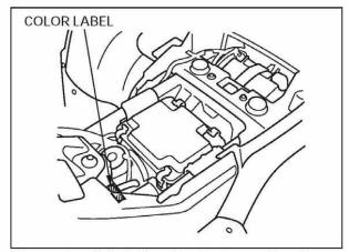
The color label is attached on the frame crossmember under the seat. When ordering color-coded parts, always specify the designated color code.
