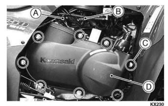
3. Remove the three cover bolts (B) in the positions shown and install an appropriate drive clutch holder (A) as shown. Note the holder's relative position to the arrow mark (D).
